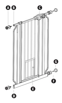
A Threaded Spindle Rods w/Adjustment Wheel Gray = #14016
